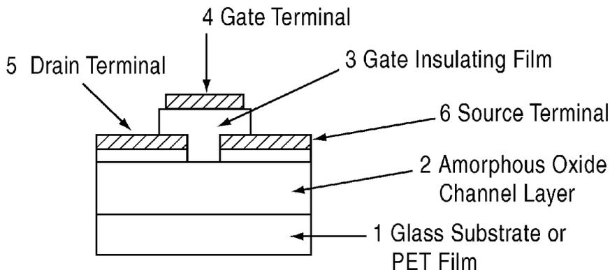
layer 2, an amorphous oxide having an electron carrier concentration less than  $10^{18}/\text{cm}^3$  is used in the channel layer 2.
