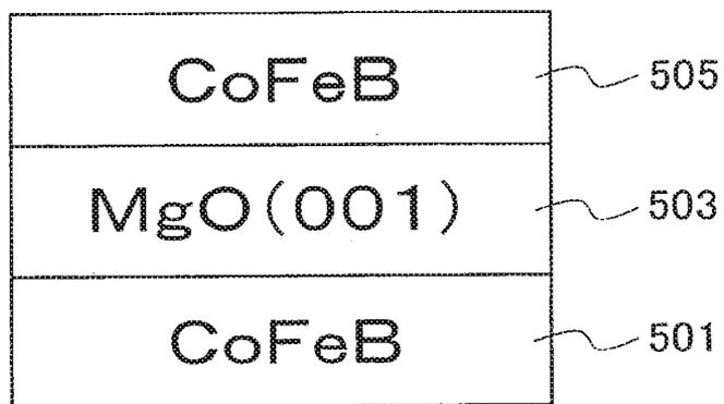
**MAGNETIC TUNNEL JUNCTION DEVICE**
