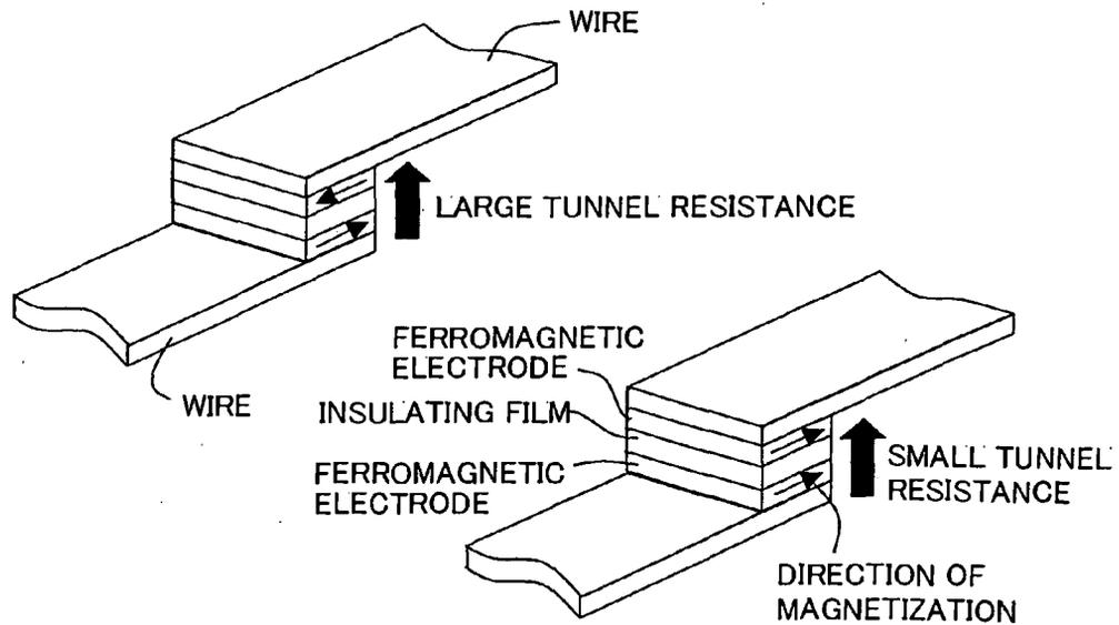
**SPIN TRANSISTOR USING SPIN-FILTER EFFECT
