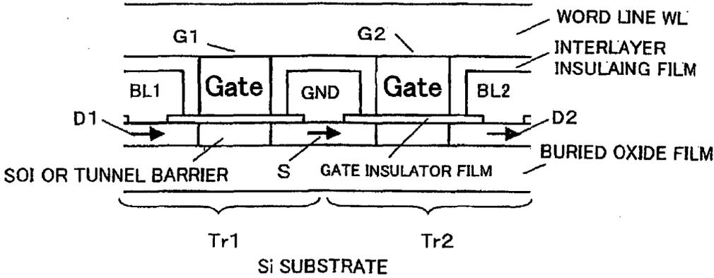
**SPIN TRANSISTOR BASED ON THE SPIN-FILTER EFFECT, AND NON-VOLATILE MEMORY USING SPIN TRANSISTORS**
