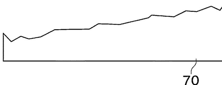
(b) SiC substrate surface after vapor-etching planarization
