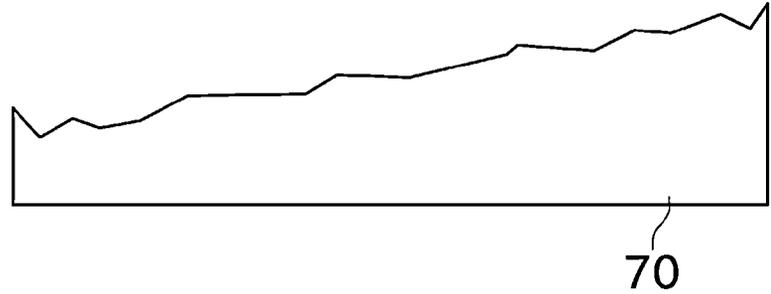
(b) SiC substrate surface after vapor-etching planarization
