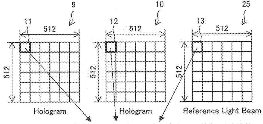
Correction Method: Compare Average Values Of Two Holograms In Identical Region, And Carry Out Calculation Of ① And ② Using Correction Value A
