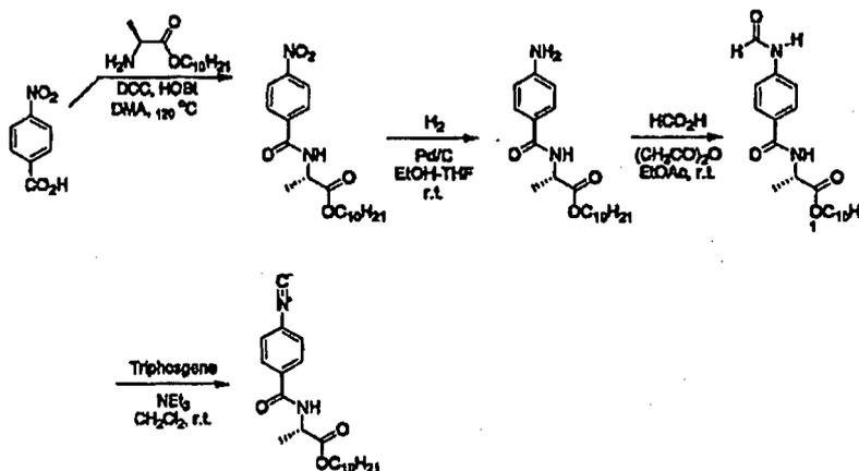
[0080] Nitrobenzoic acid was reacted with L-alanine decyl ester in t-butanol and dimethyl acetamide (DMA) in the presence of DCC as a coupling agent for amidation. Thus-obtained amide compound was reduced by a conventional reducing method so that the nitro group is reduced to an amino group. Then, it was reacted with formic acid in ethyl acetate in the presence of anhydrous acetic acid for N-formylation to give 4-formaminobenzoyl-L-alanine decyl ester.
