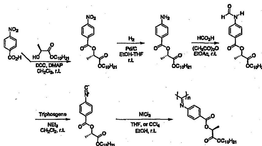
(1) Synthesis of 4-isocyanobenzoyl-L-lactic acid decyl ester as a starting monomer
