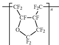
TEFLON (Registered Trademark) AF2400 and TEFLON (Registered Trademark) AF 1600 are poly[4,5-difluoro-2,2-bis(trifluoromethyl)-1,3-dioxole-co-tetrafluoroethylene], which has the following general formula:
