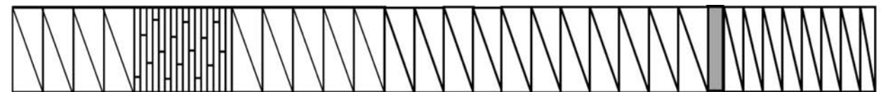
Blister screw (for PLA/CNT) : 4T-2.66K(triple thread)-0.33LK-16T-0.375B-5.16T
