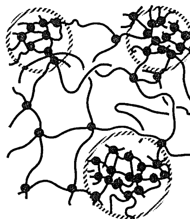
Figure 3. Speculated internal fine structures of PNIPAAm gel.
